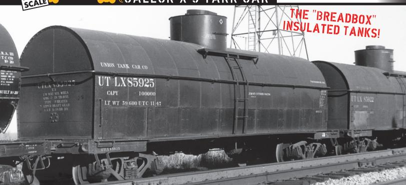
UNION TANK CAR MODIFIED A GROUP OF X-3s THROUGH THE ADDITION OF HEATER COILS OUTSIDE OF THE TANKS WITH WAGON-STYLE INSULATION AND JACKETING. THESE HIGHLY DISTINCTIVE AND INTERESTING CARS WERE PRIMARILY FOR THE TRANSPORT OF TRANSFORMER OIL, USED TO INSULATE AND COOL TRANSFORMERS. THESE CARS, NEVER BEFORE OFFERED IN STYRENE, COULD BE SEEN ANYWHERE IN THE US FROM THE 1920s INTO THE 1960s.
